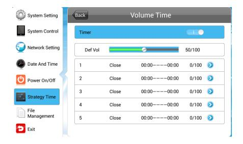
Navigate to a timer field and press "PLAY" on your remote control. Activate the timer, set a volume level and also a start and end time. Finally navigate to and select "SAVE".
