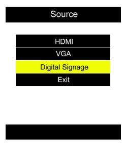
Here you can select which video signal the screen displays. As a default it is set to "Digital Signage" as this plays from the internal media player. You can also select HDMI and VGA, to do so navigate to your desired input source and press the "PLAY" button on your remote control. To go back to the previous menu navigate to Return and press "PLAY" on your remote control.
