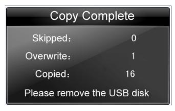
6. The unit will now restart (if it doesn't please turn off and back on via the mains) and play the stored files in a loop on both sides of the display.
